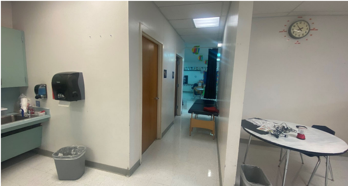
Studios configured with a connected corridor to connected restrooms. Connection allows sound to pass from one studio to the next.
